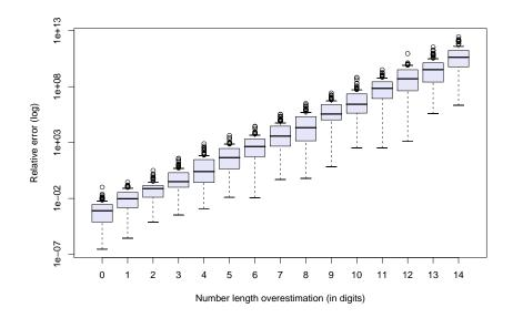
Fig. 3. Relative error obtained after 1000 fitness evaluations with an overestimated (in this case aimed at 15 digits) exact-length grammar. Note the logarithmic scale in the error axis.
