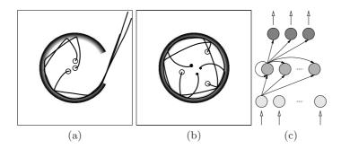
**Fig. 2.** (a,b) The experimental arena contains a circular band in shades of grey, which may or may not have the *way out*. Dark lines represent the trajectory of three *s-bots*, and the starting position on the trajectories is indicated by empty circles. (c) The three-layer architecture of the neural controller. The hidden layer is composed of continuous time neurons with fully recurrent connections.
